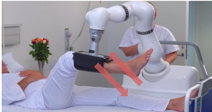
Figure 4.3: The path in which ROBERT will move the leg. (Life Science Robotics 2019)
