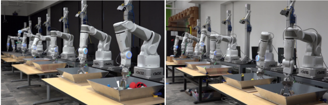
Figure 2.1: A setup with fourteen robots used by Levine et al. (2016) to collect 800,000 grasps.
