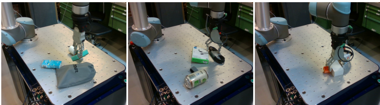
Figure 6.8: Examples of failed attempts. The most common cause of failure is obstruction of a finger by another object, which prevents the RG2 gripper from closing.
